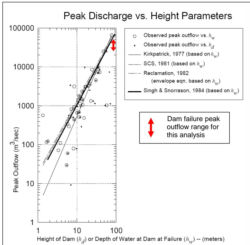
**Figure 8: Peak Discharge vs. Height for observed dam failures (Wahl, 1998)**
