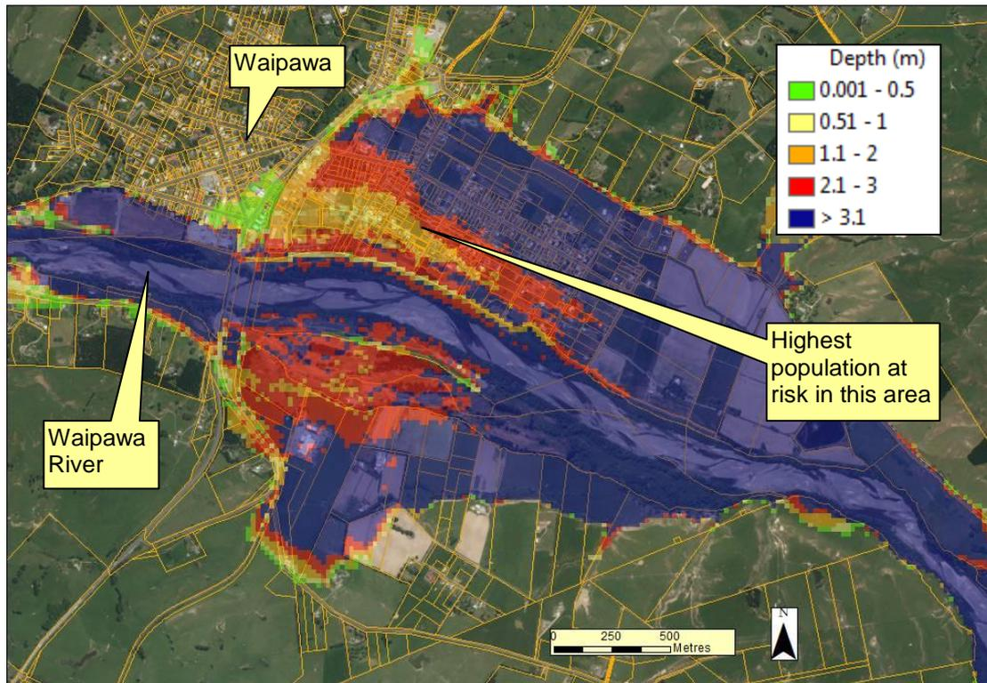
**Figure 34: Waipawa, showing properties to indicate population-at-risk, sunny day failure, 45,000 m<sup>3</sup>/s**
