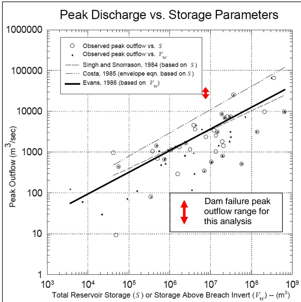
Figure 9: Peak Discharge vs. Storage Parameters for dam failures (Wahl, 1998)
