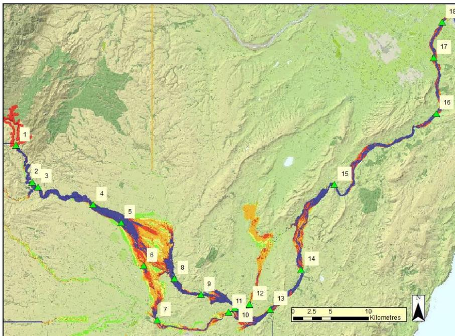
Figure 28: Flood extent results for sunny day failure, 45,000 m<sup>3</sup>/s scenario
