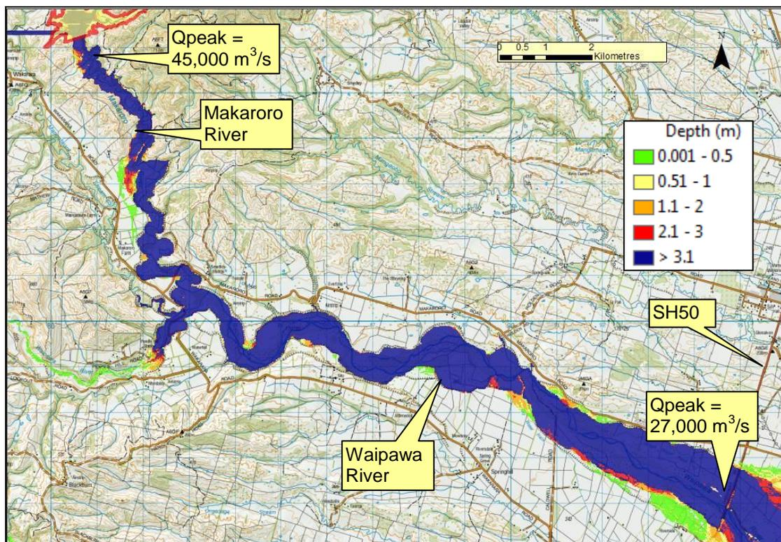
Figure 15: Makaroro River and Waipawa River to SH50, flood depths for sunny day failure, 45,000 m<sup>3</sup>/s
