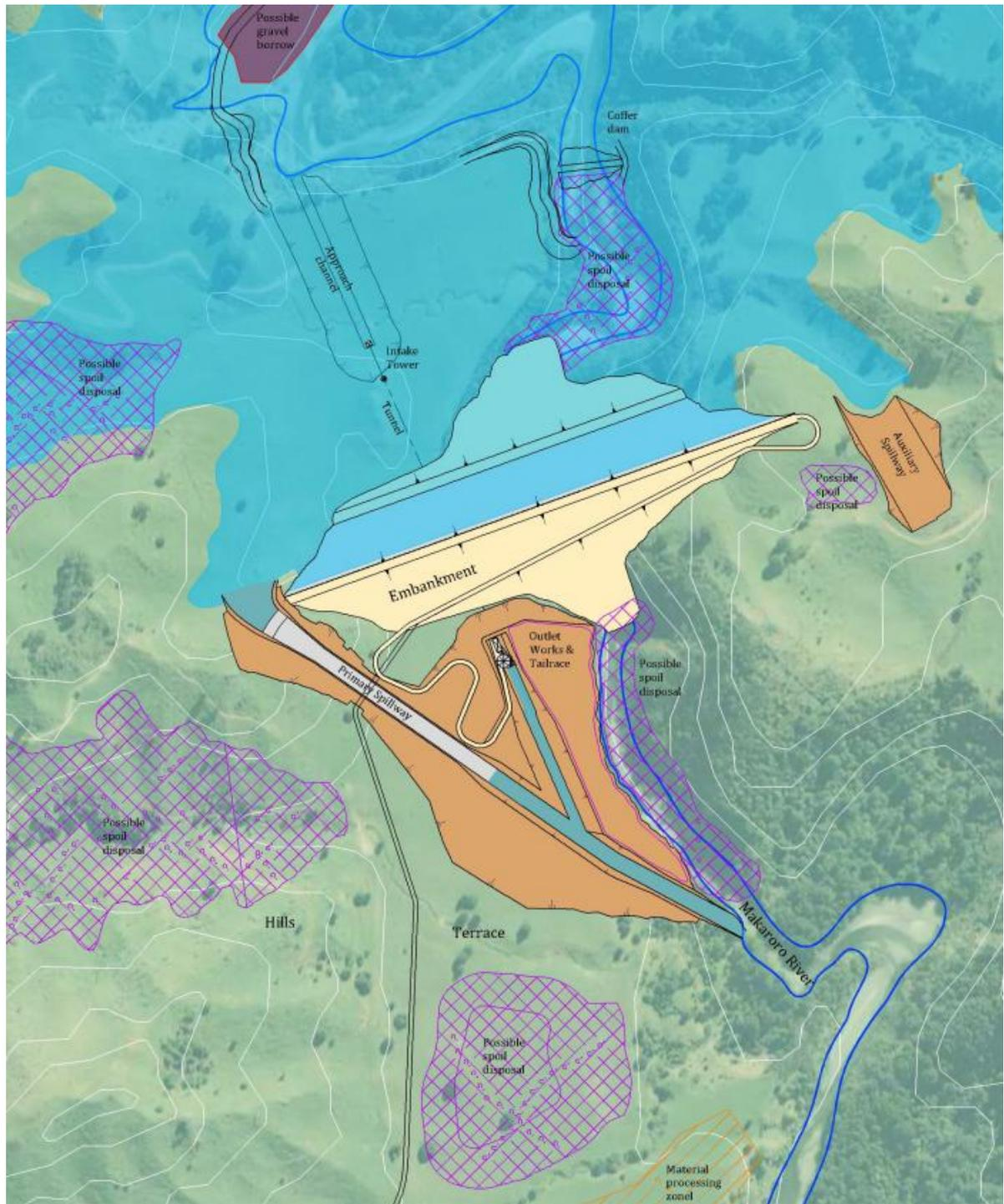
Figure 2: Layout of proposed dam
