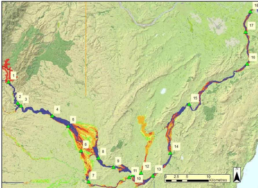
Figure 27: Flood extent results for sunny day failure, 25,000 m<sup>3</sup>/s scenario
