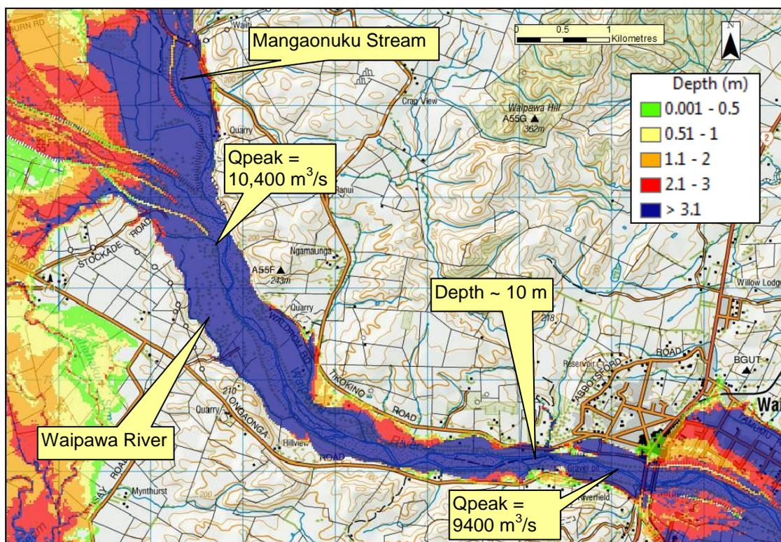
Figure 19: Waipawa River, Mangaonuku Stream to SH2, flood depths, sunny day failure, 45,000 m<sup>3</sup>/s
