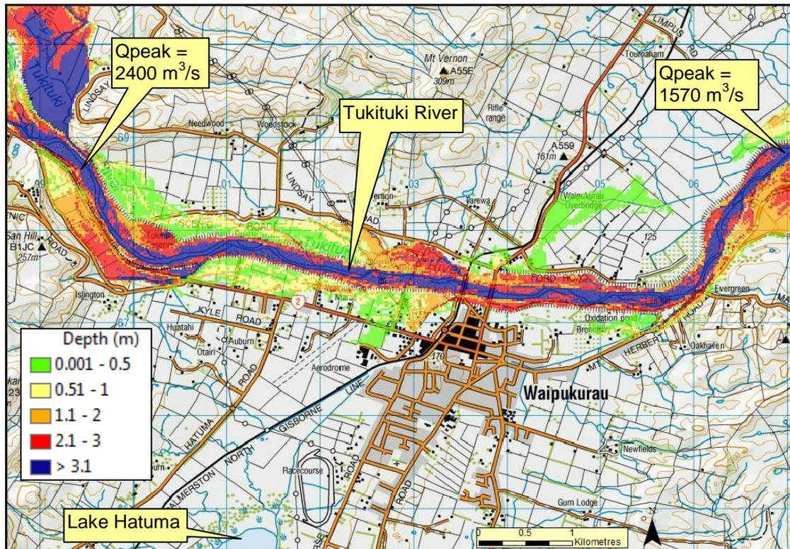
Figure 18: Tukituki River at Waipukurau flood depths, sunny day failure, 45,000 m<sup>3</sup>/s
