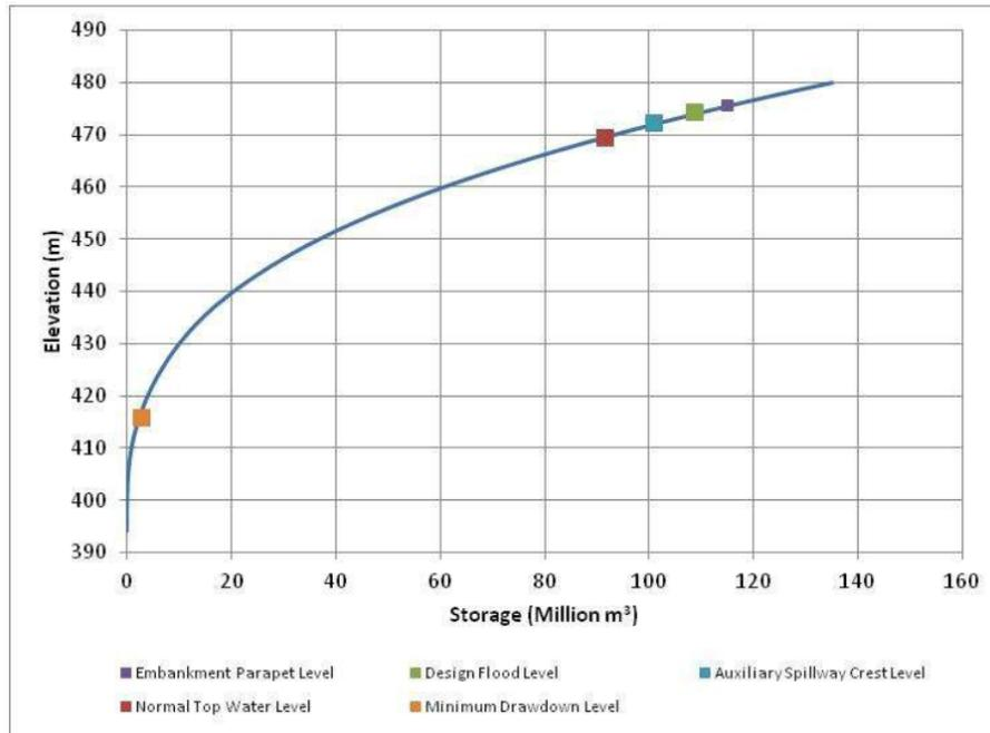
Figure 5: Storage elevation curve for proposed dam
