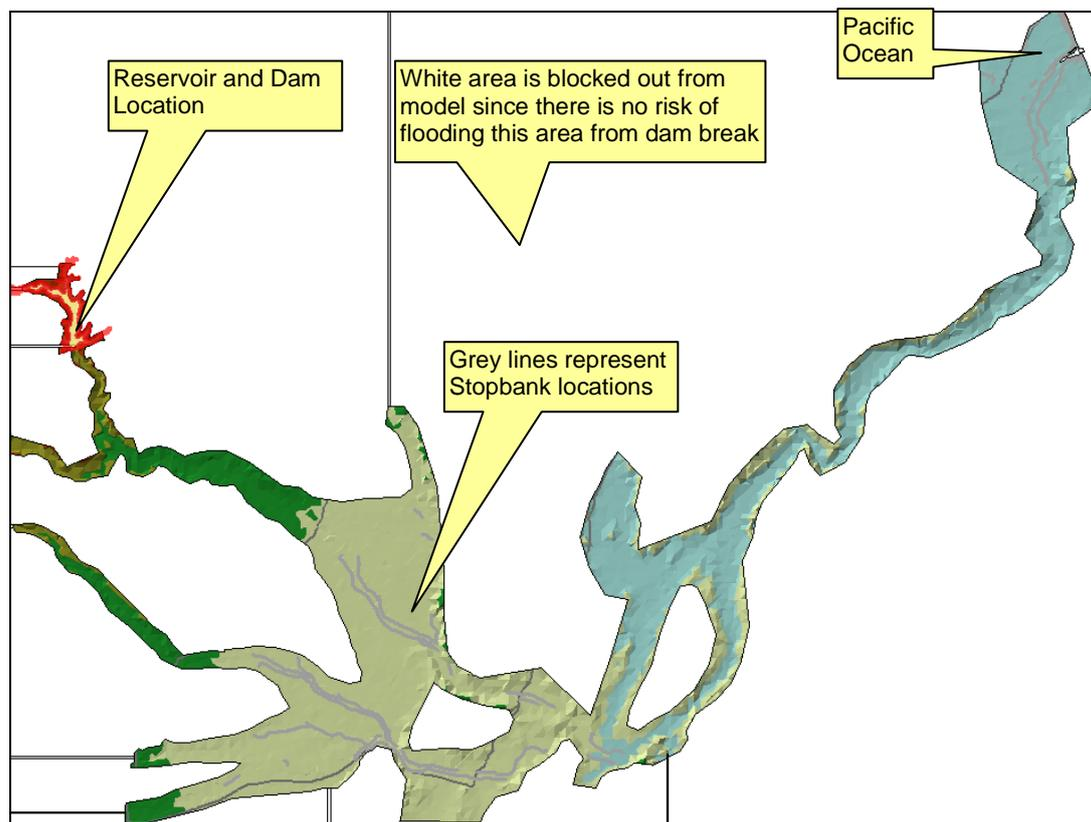
Figure 11: Digital Elevation Model used in 2D Hydrodynamic Model.
