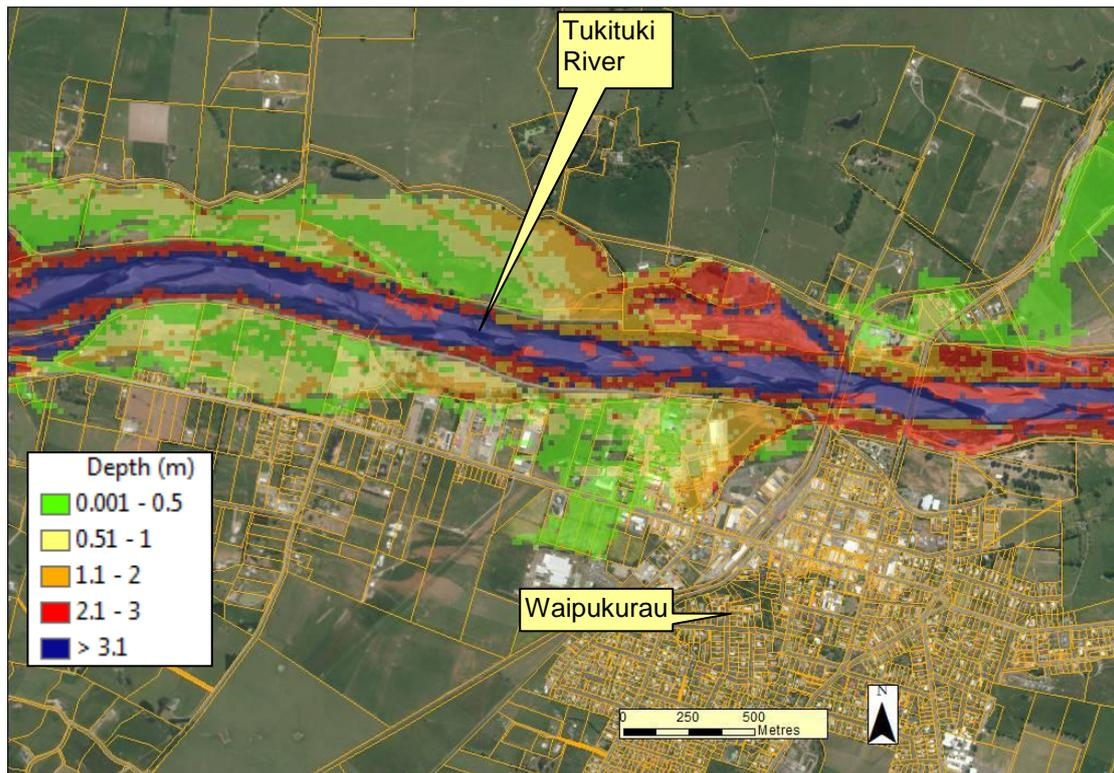
**Figure 35: Waipukurau, showing properties to indicate population-at-risk, sunny day failure, 45,000 m<sup>3</sup>/s**
