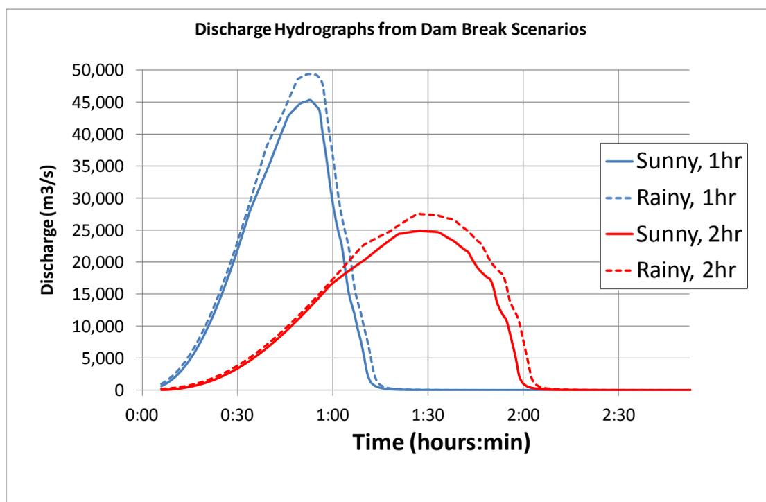
Figure 7: Discharge hydrographs from dam break model.
