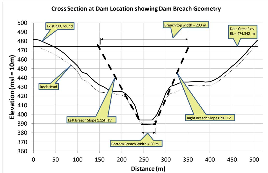
Figure 6: Cross-Section at dam location showing dam breach geometry
