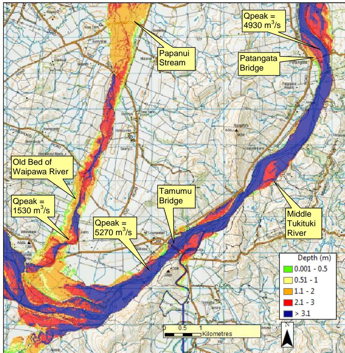
Figure 21: Papanui, Tukituki River flood depths, sunny day failure, 45,000 m<sup>3</sup>/s
