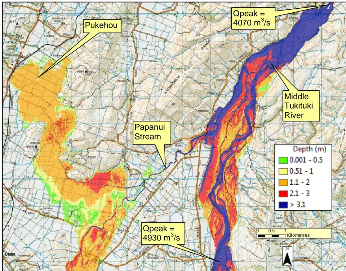
Figure 22: Papanui/Pukehou flood depths, sunny day failure, 45,000 m³/s
