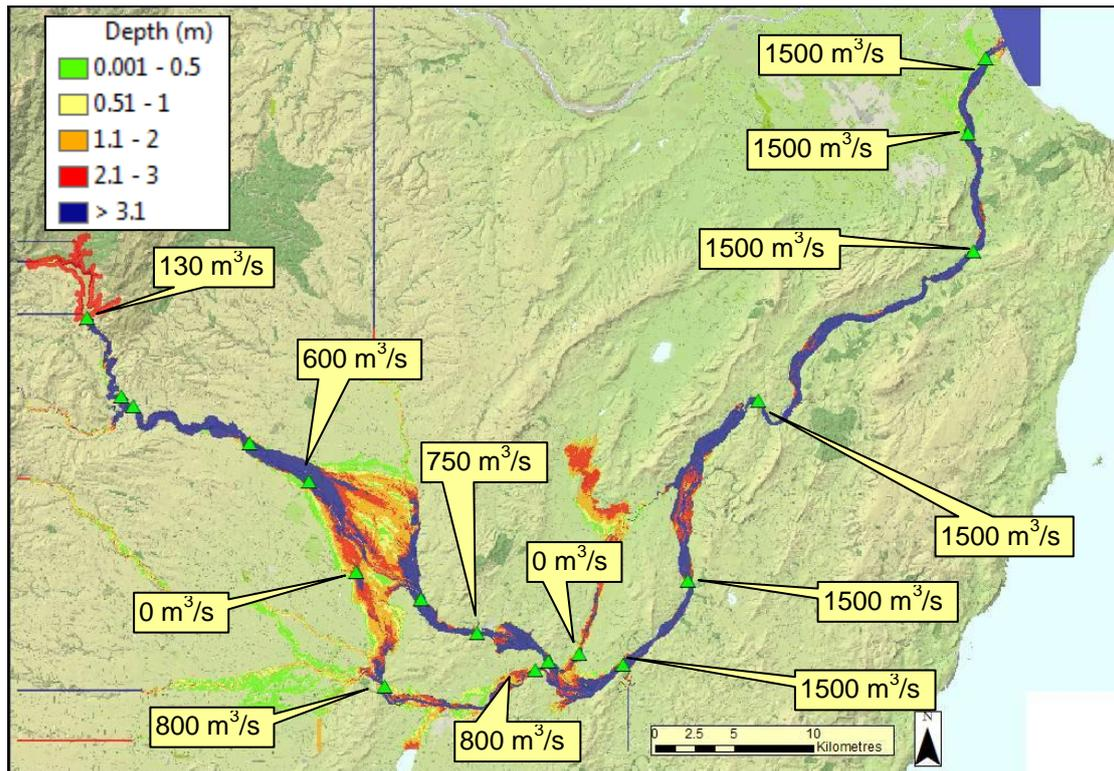
**Figure 30: Constant discharge values in rivers for rainy day failure, 49,000 m<sup>3</sup>/s scenario**
