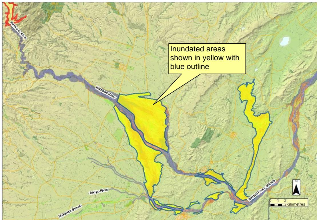
**Figure 26: Inundated area outside of normal flood risk area on rivers, sunny day failure, 45,000 m<sup>3</sup>/s scenario.**
