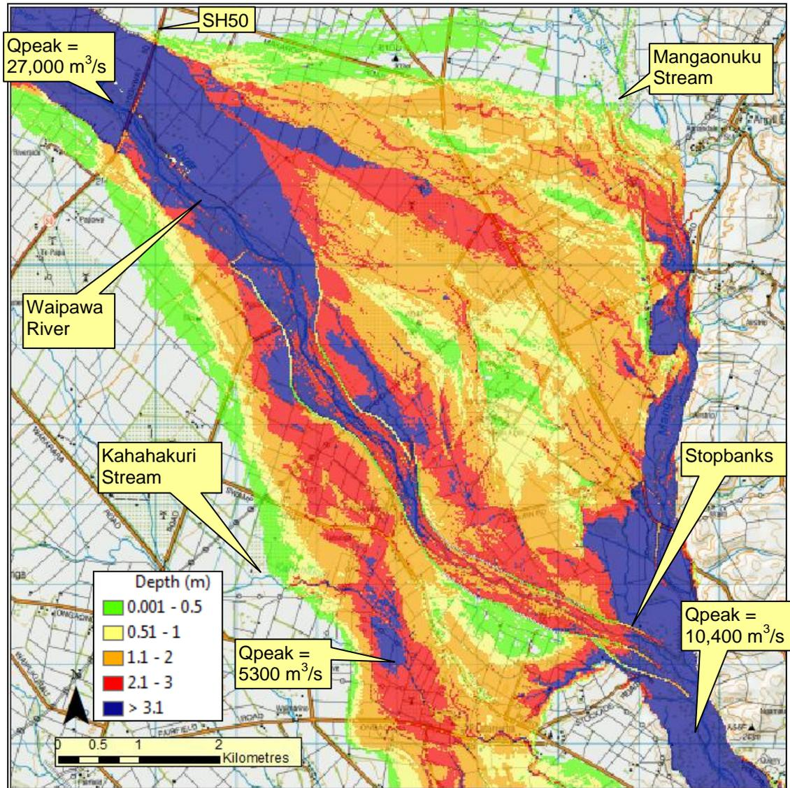
Figure 16: Waipawa River downstream SH50 for sunny day failure, 45,000 m<sup>3</sup>/s
