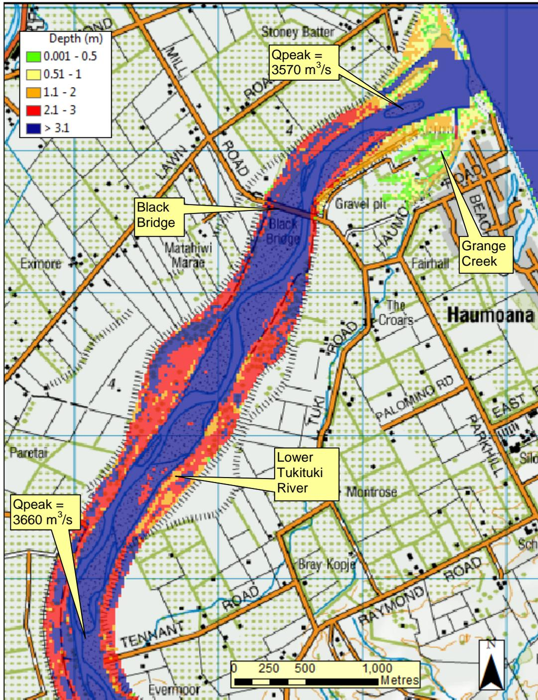
Figure 25: Lower Tukituki River flood depths, sunny day failure,  $45,000 \text{ m}^3/\text{s}$
