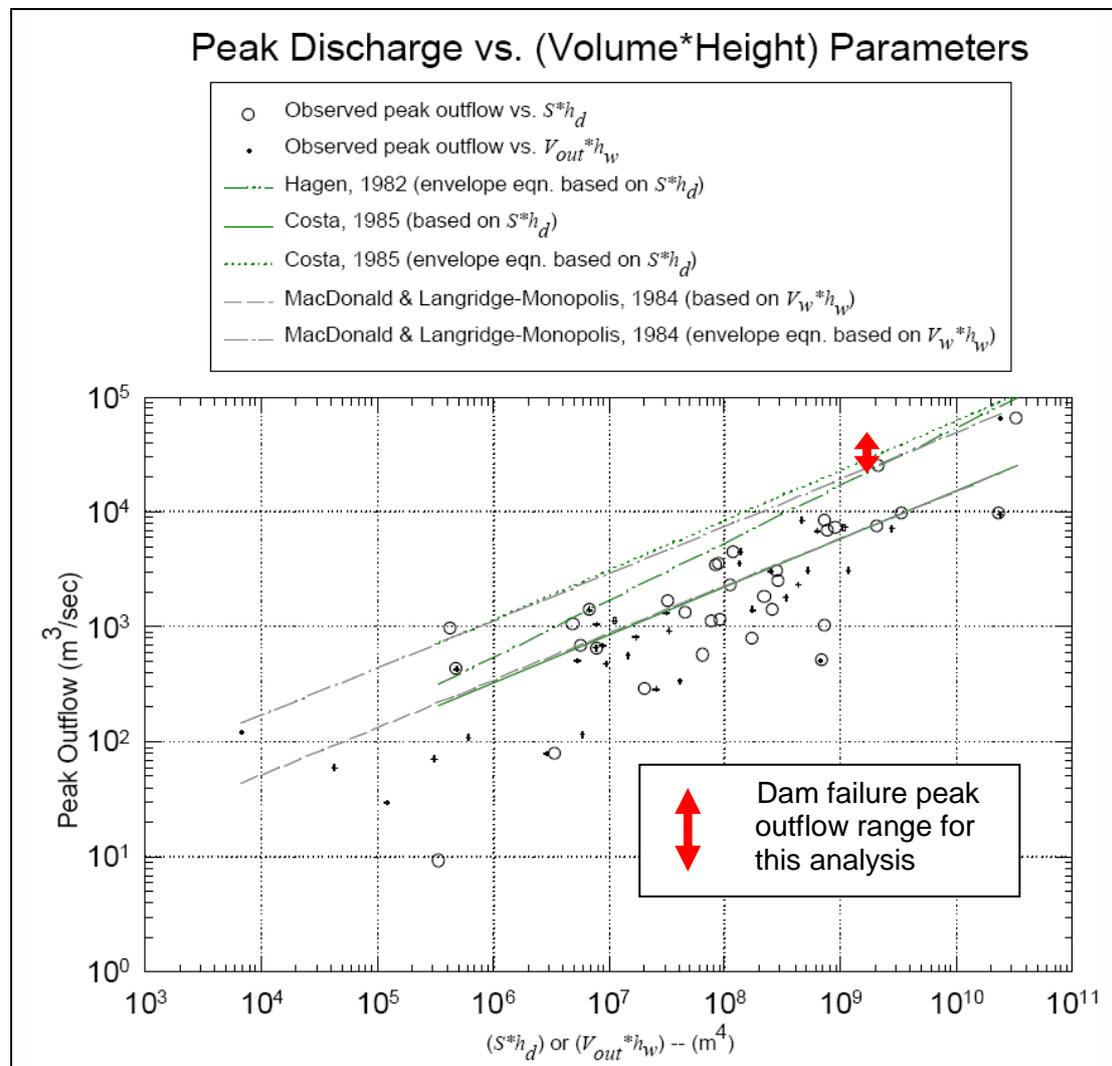
Figure 10: Peak Discharge vs. (Volume x Height) for dam failures (Wahl, 1998)
