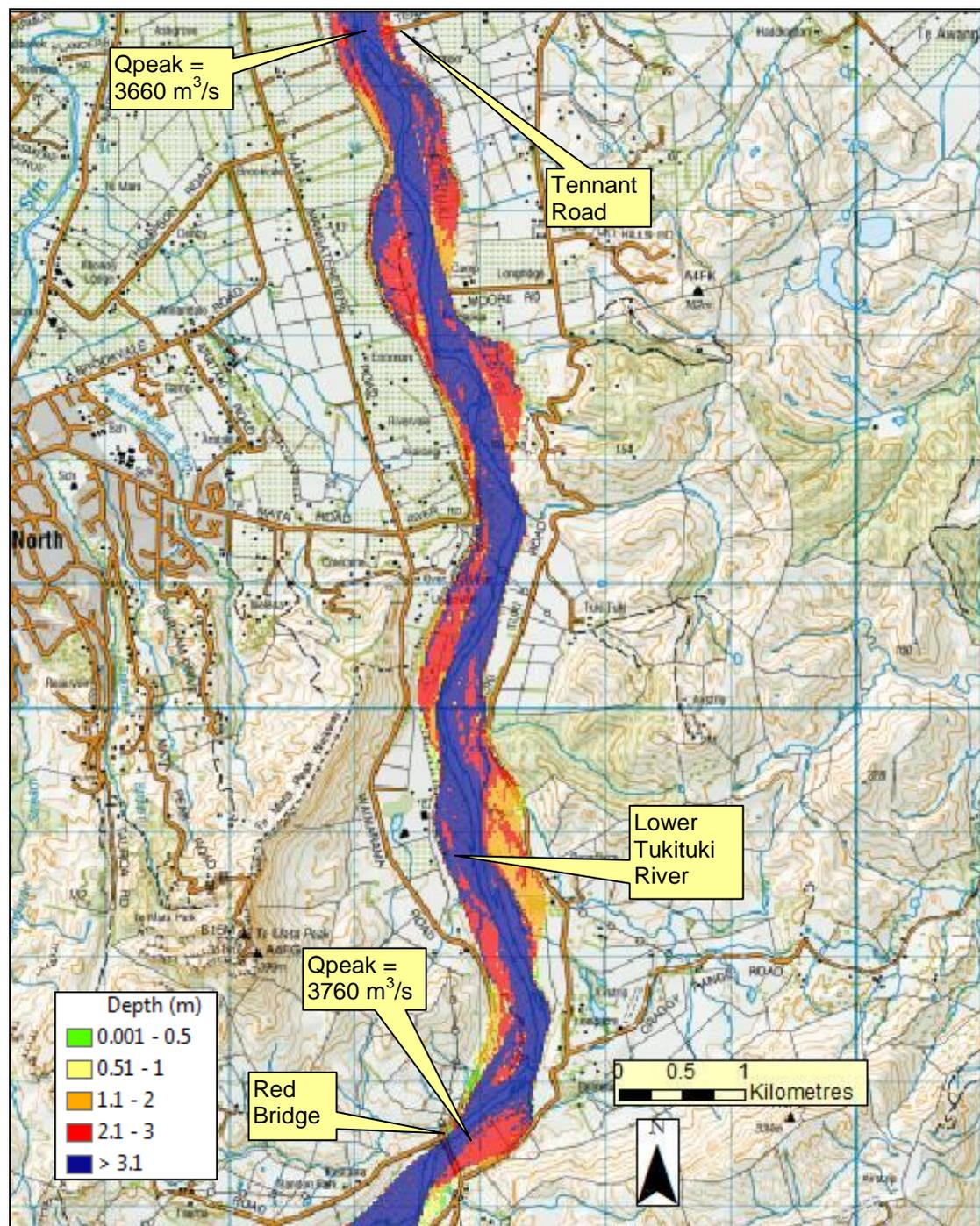
Figure 24: Tukituki River near Red Bridge, flood depths, sunny day failure,  $45,000 \text{ m}^3/\text{s}$
