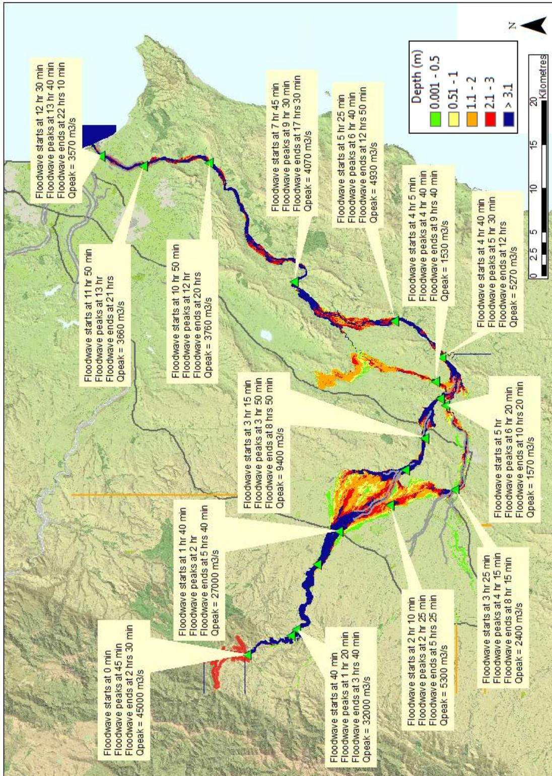
Figure 12: Timing and discharge results for sunny day failure, 45,000 m<sup>3</sup>/s scenario
