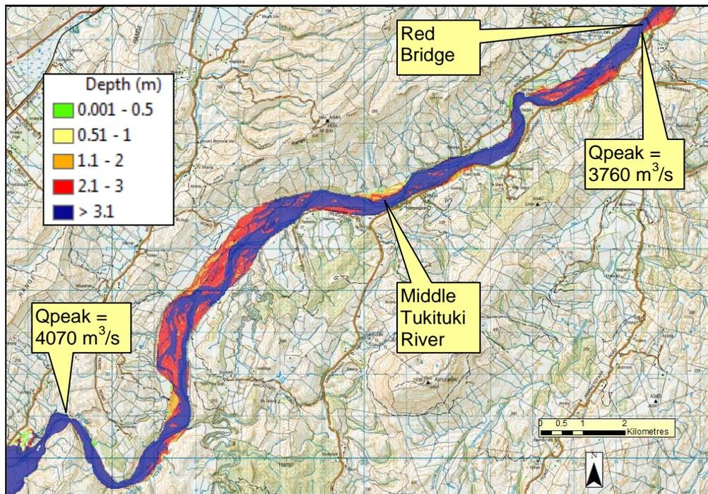
Figure 23: Middle Tukituki River flood depths, sunny day failure, 45,000 m³/s
