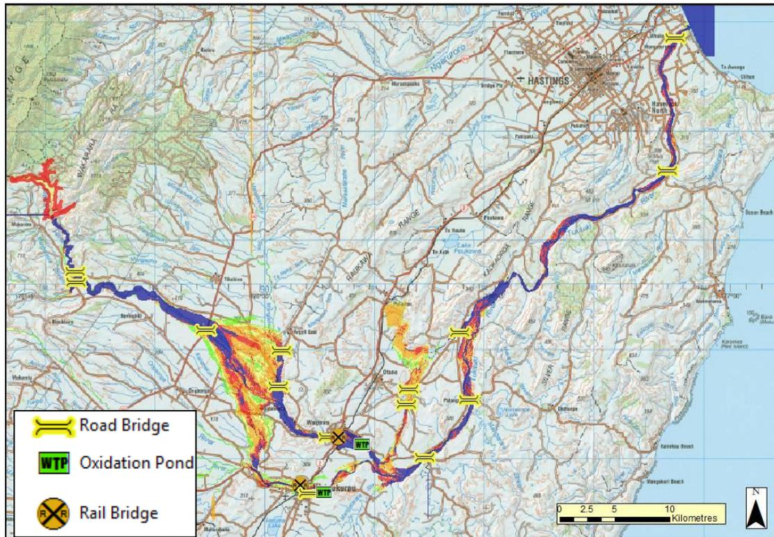
**Figure 33: Locations of bridges or infrastructure at risk, sunny day failure, 45,000 m<sup>3</sup>/s**
