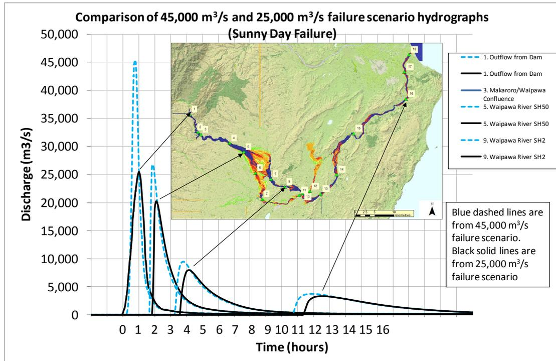
**Figure 29: Discharge hydrograph comparison for 45,000 m<sup>3</sup>/s and 25,000 m<sup>3</sup>/s scenario, sunny day failure**
