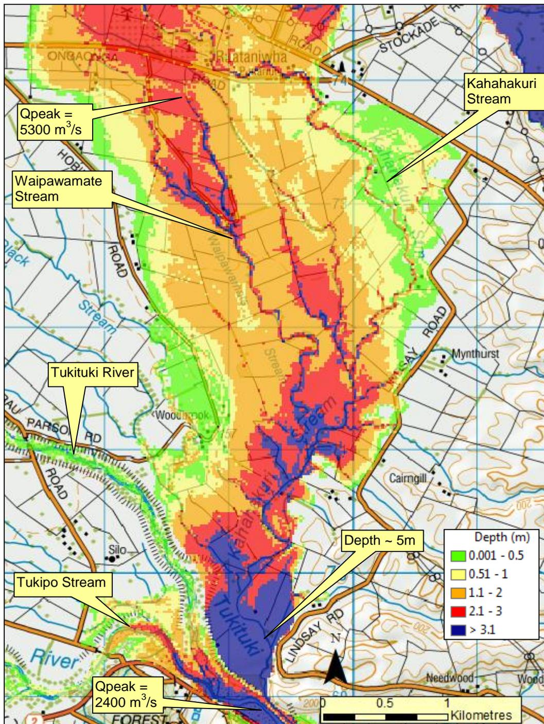
Figure 17: Kahahakuri and Waipawamate flood depths, sunny day failure,  $45,000 \text{ m}^3/\text{s}$
