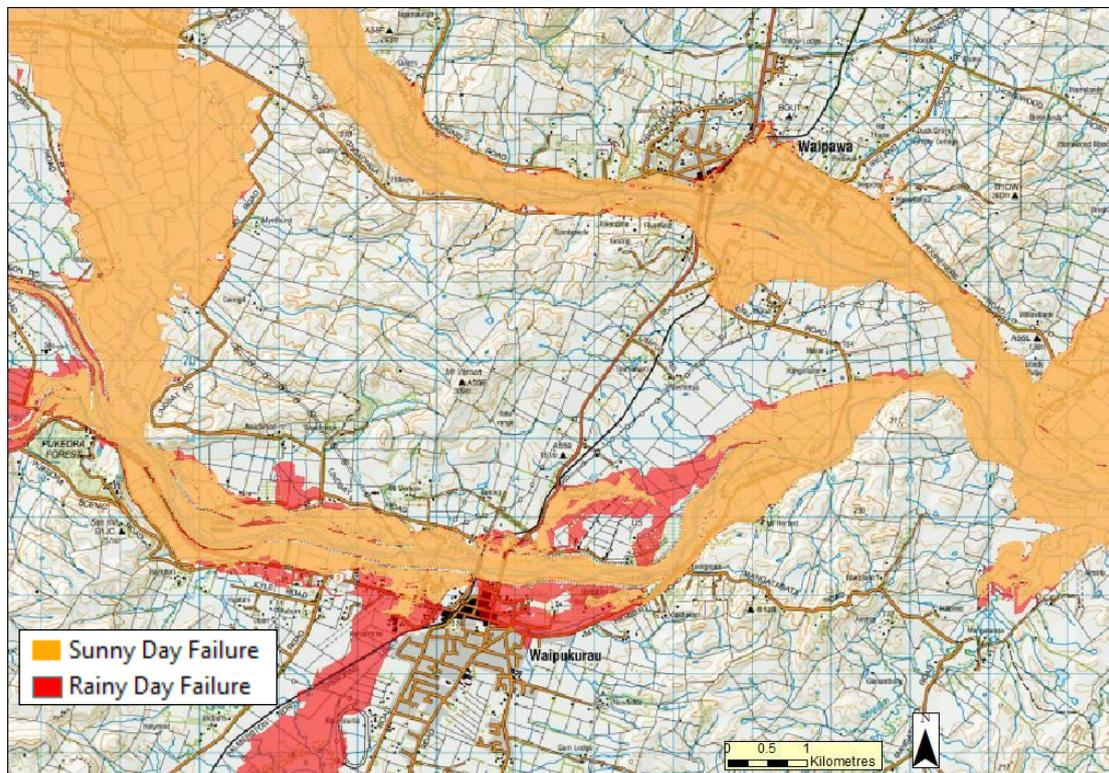
**Figure 32: Differences between sunny and rainy day failures (both 1-hour failure scenarios)**
